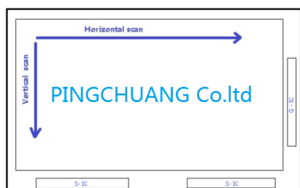
Fig. 1 Normal scan (Pin24, Reverse = Low or NC)
